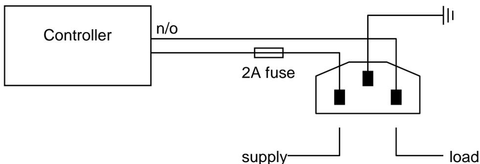
The purpose of the 2 amp fuse is to guard against the connection of a mains supply to the panel plug.
